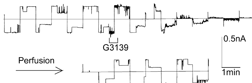
Fig. 5 A single VDAC channel reconstituted into a planar phospholipid membrane is closed by G3139. The voltage was alternated every 50 s between +50 and -50 mV to show VDAC gating. The zero current level is indicated as a long horizontal line. G3139 (40 \mu\text{M} final) was added where indicated. The side of the membrane
